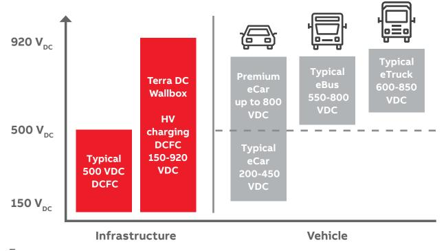
A high range of DC voltage capability is demanded to deliver efficient charging services to every EV and use case.
