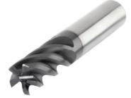
The WCE5 5-flute geometry combines the unequal index feature with an elevated 38-degree helix feature at an affordable price. WCE5 can be used primarily in carbon steel and stainless steels shouldering/side milling applications.
